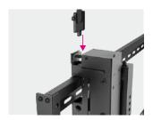
Pop-out Lock System ensures safety use by reducing the possibility of accidental pop-outs via the additional plastic plug-in pieces.
